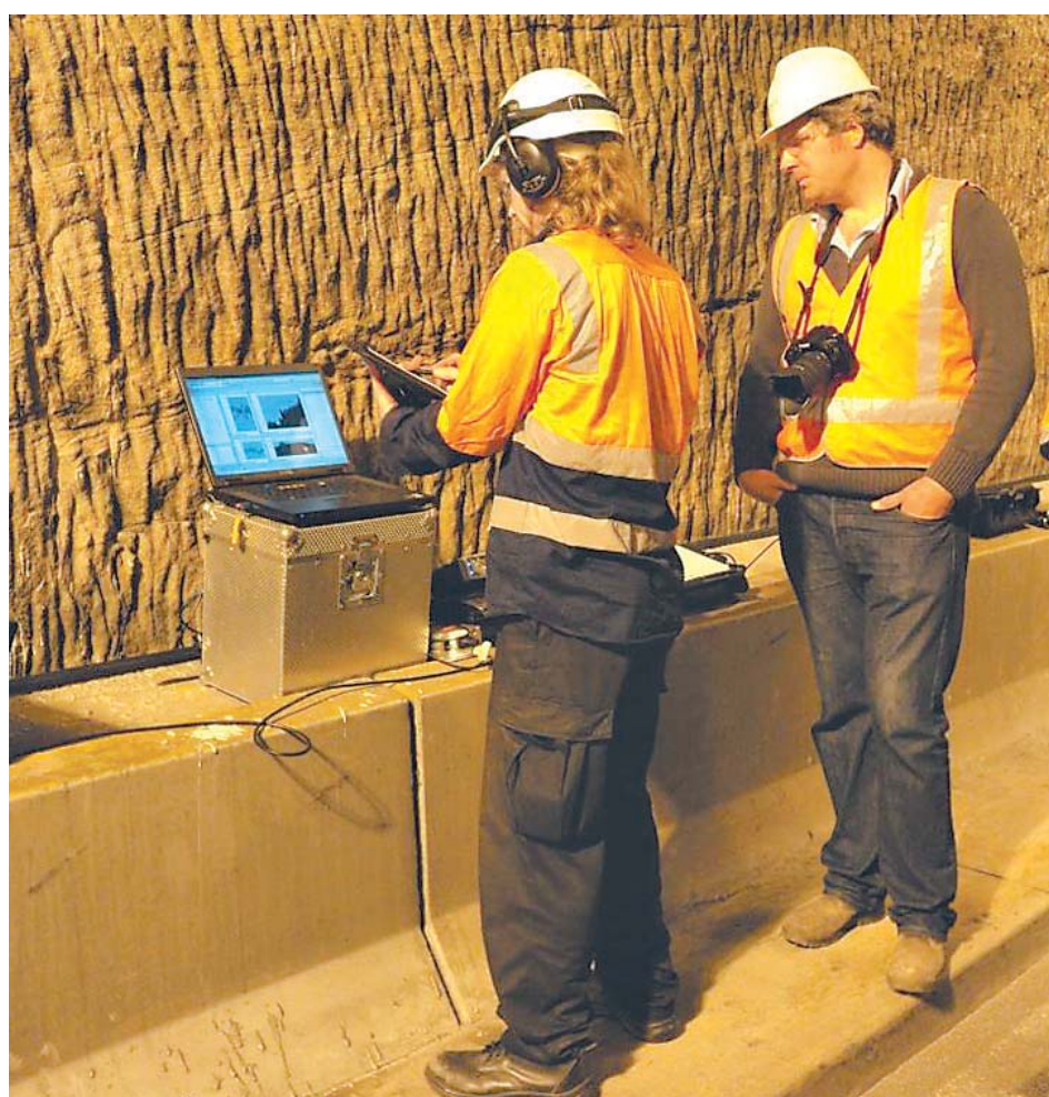
Vibration monitoring equipment in the tunnel.
